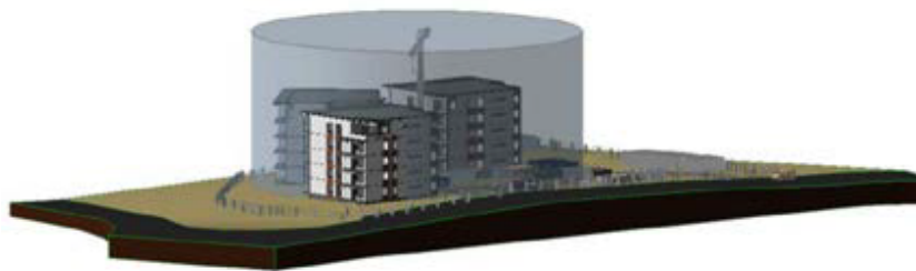
Figure 4.5 Visualization of crane swings (Khoshnava et al., 2012)
